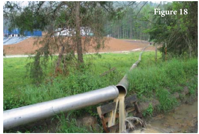
An open pipe leading from a drilling pad discharges into a ditch. The contents of drilling waste is not disclosed to the public.
