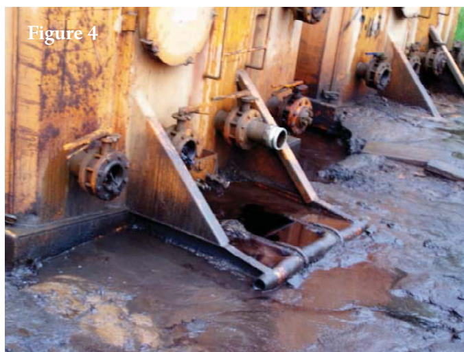
Drilling mud, which can contain natural gas and other flammable materials, leaking from tanks at a land farm that has since been shut down.
