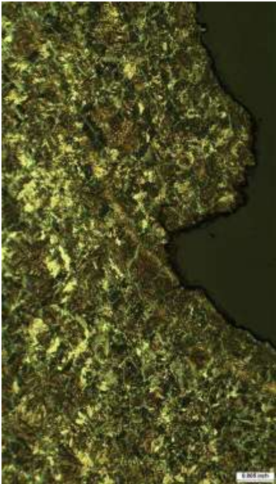
20' 6-13/16" from the North Girth Weld 2% Nital etch, ~100x Photograph No. 181
