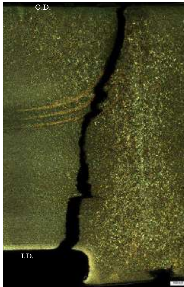
20' 4-7/8" from the North Girth Weld 2% Nital etch, ~25x Photograph No. 160
