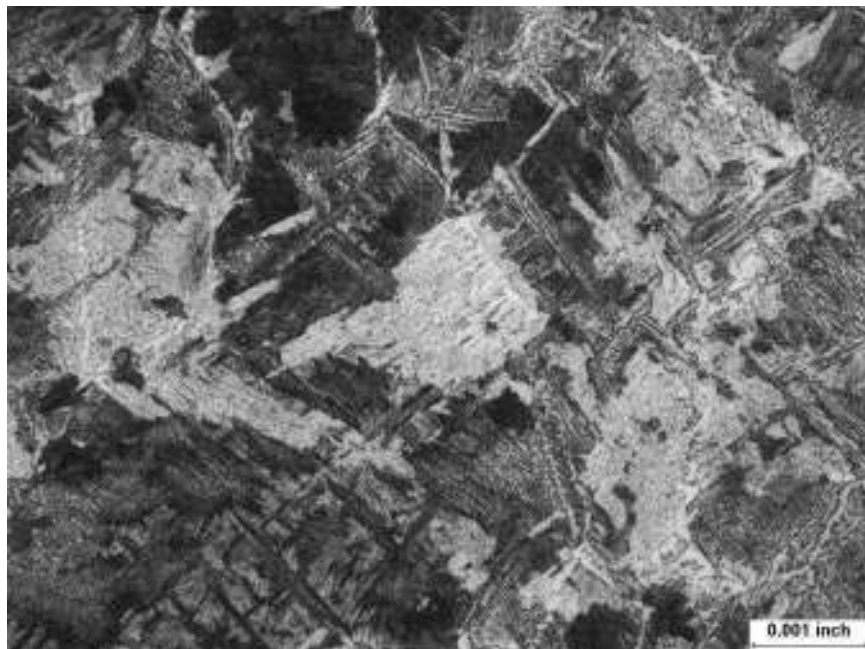
Fusion Line 2% Nital etch, ~100x Photograph No. 193
