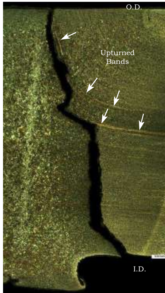
20' 6-13/16" from the North Girth Weld 2% Nital etch, ~25x Photograph No. 178
