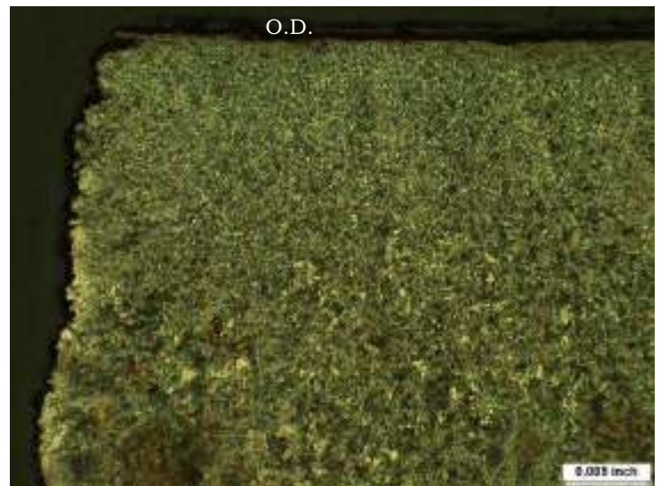
20' 6-13/16" from the North Girth Weld 2% Nital etch, ~100x Photograph No. 180
