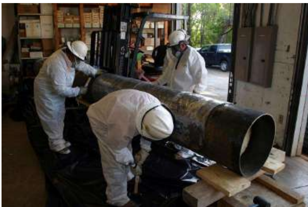
The photographs display the coating removal that was carried by impacting with steel or composite hammers.
