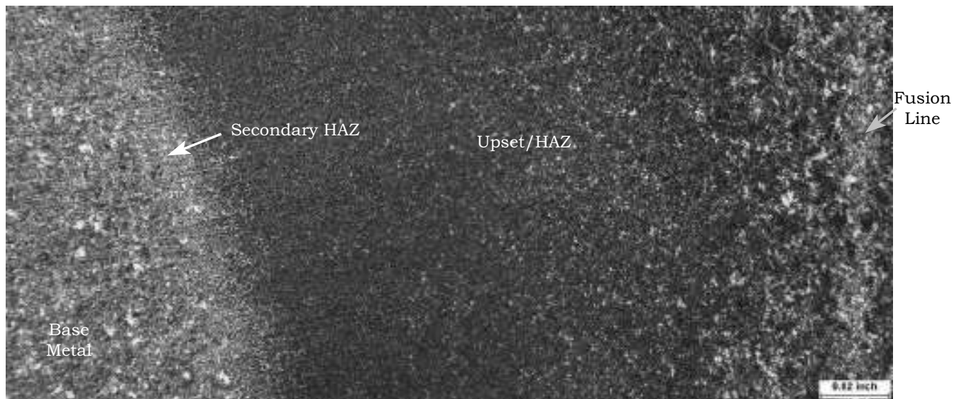
Fusion Line to Base Metal 2% Nital etch, ~25x Photograph No. 191
