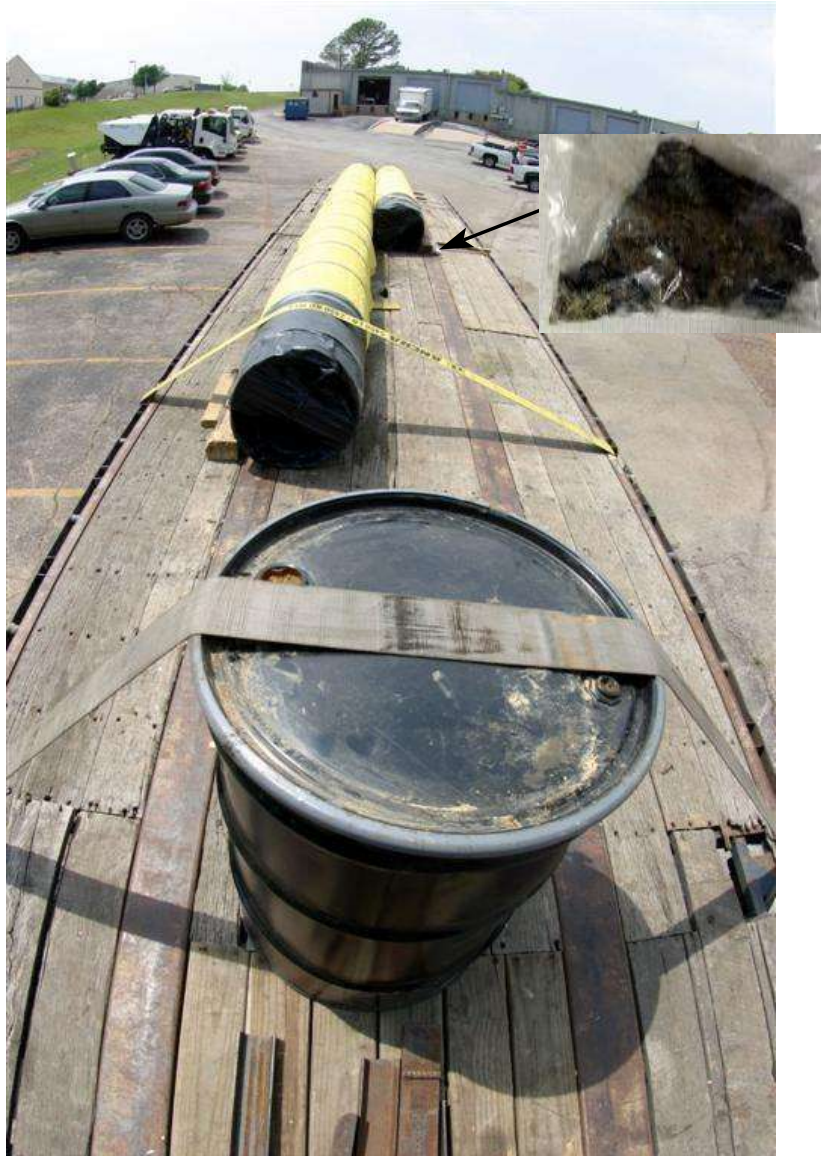
The photograph displays the pipe section, a drum containing the coating material that was removed in the field prior to sectioning of the cracked pipe and a bag containing possible calcareous deposit.
