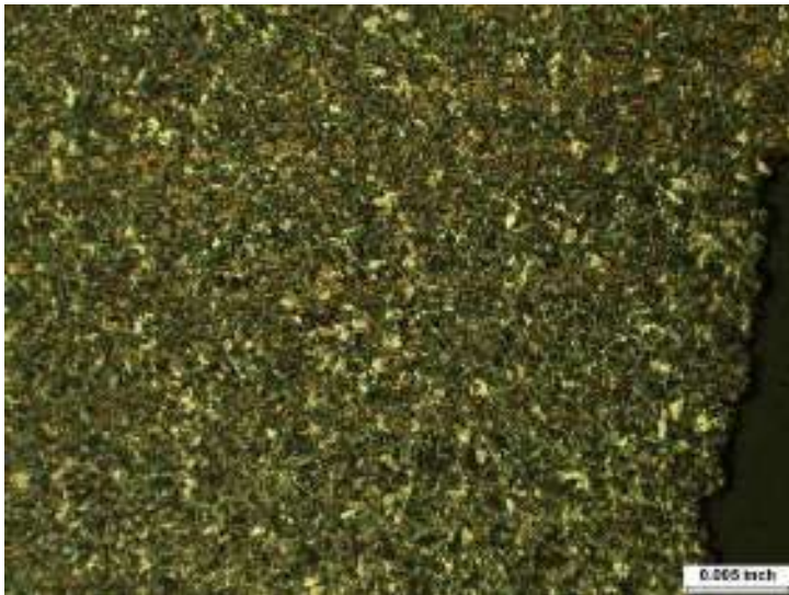
20' 4-7/8" from the North Girth Weld 2% Nital etch, ~100x Photograph No. 165
