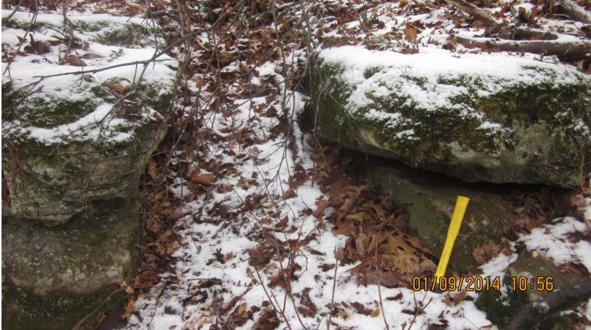
Photo 7. Limestone outcrop with solution enhanced bedding plane and fracture forming an open fissure (SE-03 on Figure 2.1).
