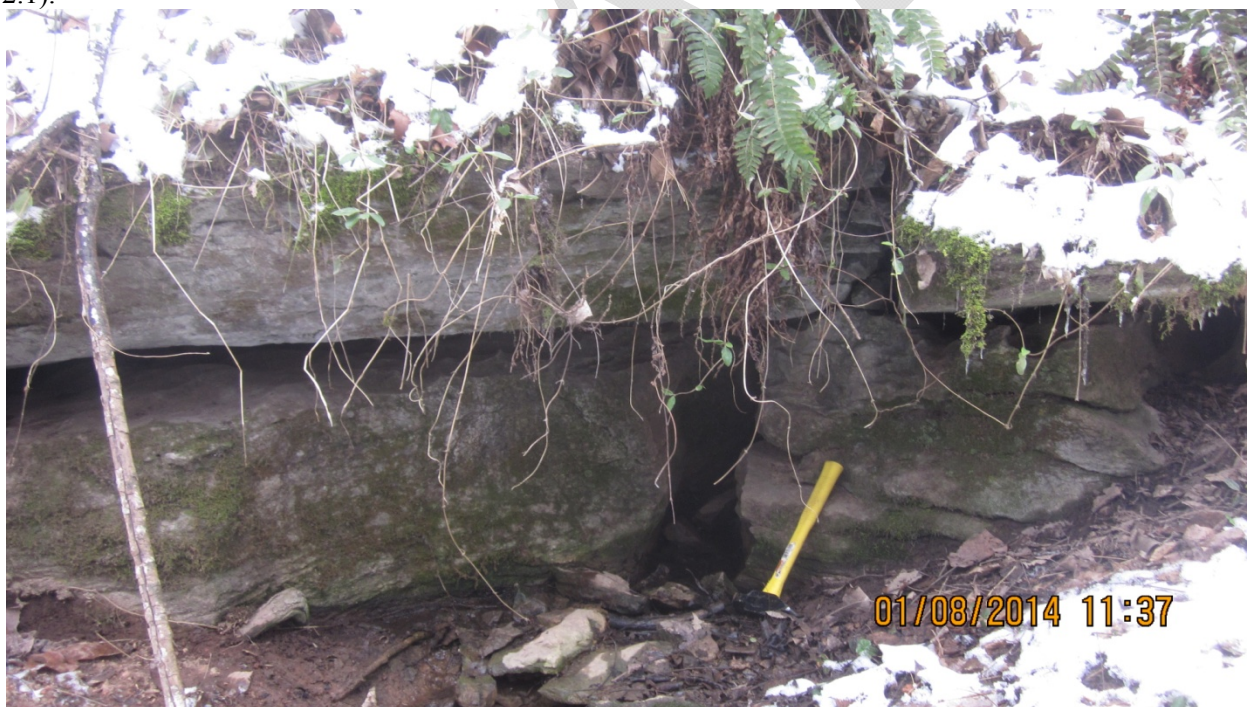
Photo 2. Limestone outcrop of Boone Formation with solution enhanced bedding planes and fracture. Spring emerges from base of fracture (SW-05 on Figure 2.1).
