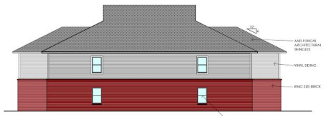
BUILDING #4 - SOUTH ELEVATION 1/8" = 1'-0"
