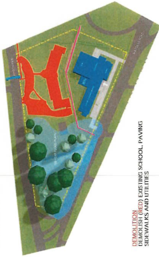
EXISTING SITE / DEMOLITION DEMOLISH (RED) SECTIONS OF EXISTING PAVING, ACCESSORY STRUCTURES AND CLASSROOM WING TO ACCOMMODATE NEW CONSTRUCTION
